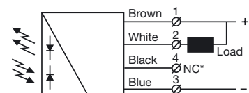
*Do not connect black wire SMP/SMPF/SMRR 7600 (load as NPN)
